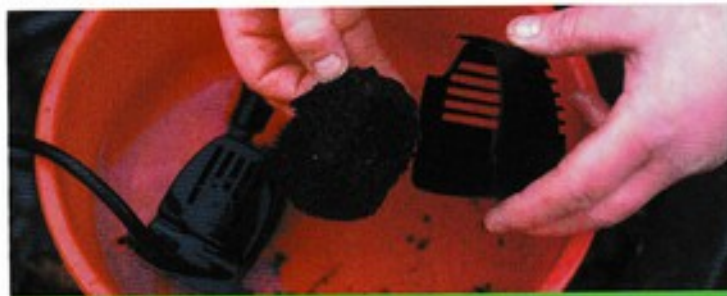
Pre-filters tend to be relatively small and will clog quickly. This causes the flow rate to drop dramatically which affects the efficiency of your filter. To prevent this happening you have to clean your pre-filter frequently.
